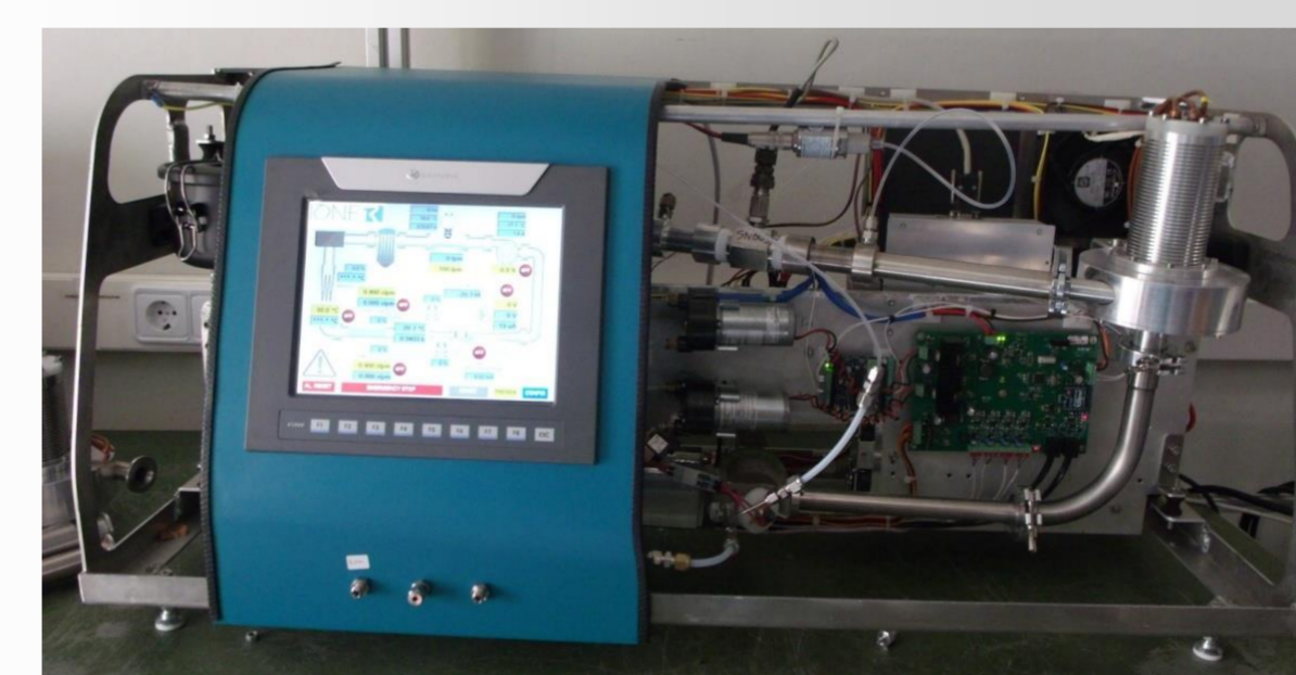
prototype of HR-SMPS instrument for very small particles
