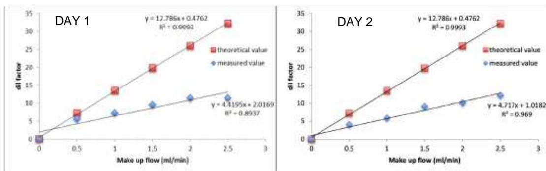
Figure 3: The accuracy of the interface prototype split ratios for fluorescein (first set up).
