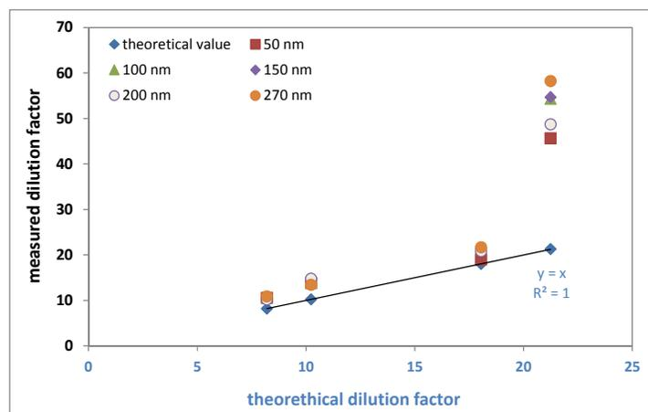
**Figure 5:** The accuracy of the interface prototype for PSS of different size (second set up).
