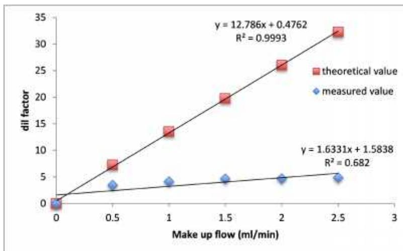
Figure 4: The accuracy of the interface prototype split ratios for PSS100 (first set up).
