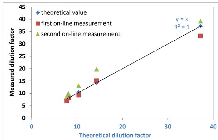
Figure 7: Calculated and measured interface prototype dilution factors.
